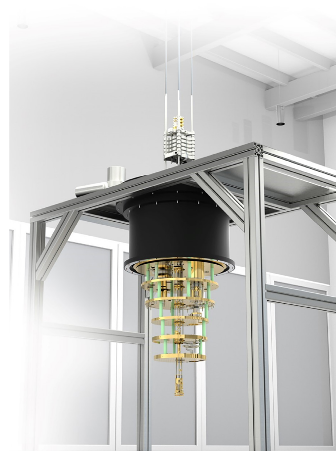
Figure 1: Typical depiction of a quantum computer: a cryostat. It cools the quantum processor down to a few milli Kelvin.
