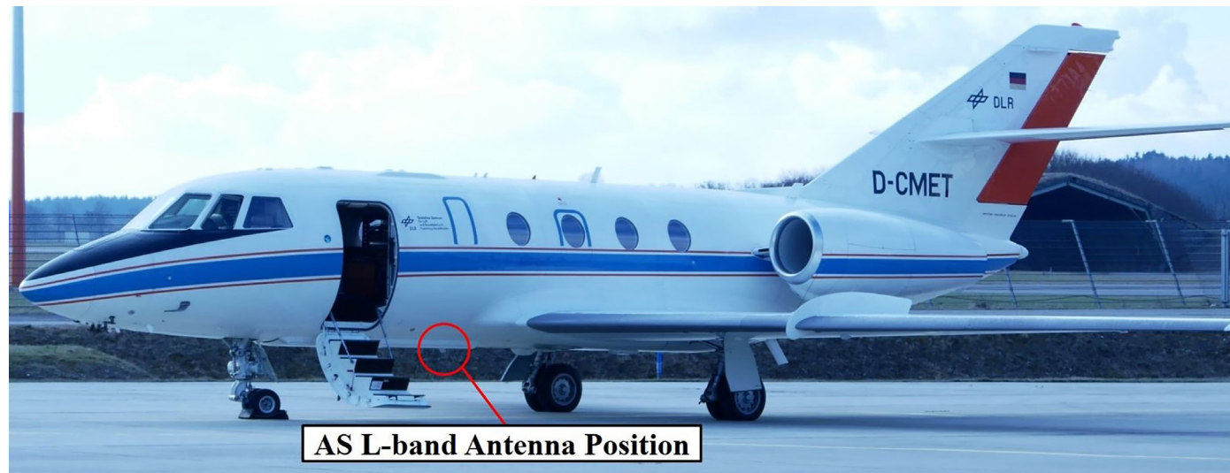
Figure 4: DLR's research aircraft Dassault Falcon 20E (D-CMET) used in the experiments. [23]
